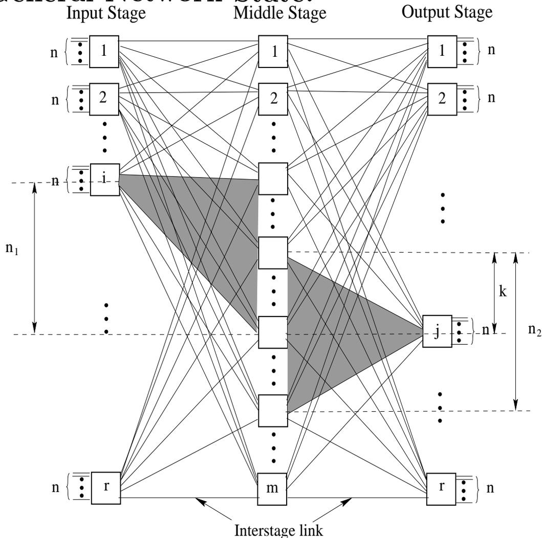
A three-stage Clos network with  $n_1$  busy input-middle interstage links from input stage switch  $i$ ,  $n_2$  busy middle-output interstage links to output stage switch  $j$ , and  $k$  pairs of the interstage links overlapped.
