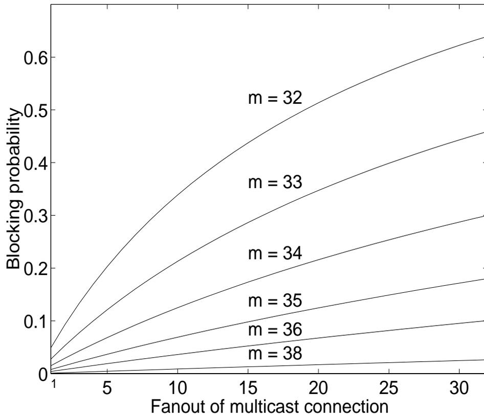
The blocking probability  $P_B(f)$  is an increasing sequence of fanout  $f$ .
