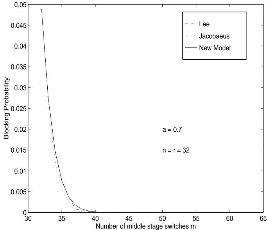
The blocking probabilities of the Clos network in three models: Lee, Jacobaeus and the new model, for a network with  $n = r = 32$  and  $n \leq m \leq 2n - 1$ , under network input link utilization  $a = 0.7$ .
