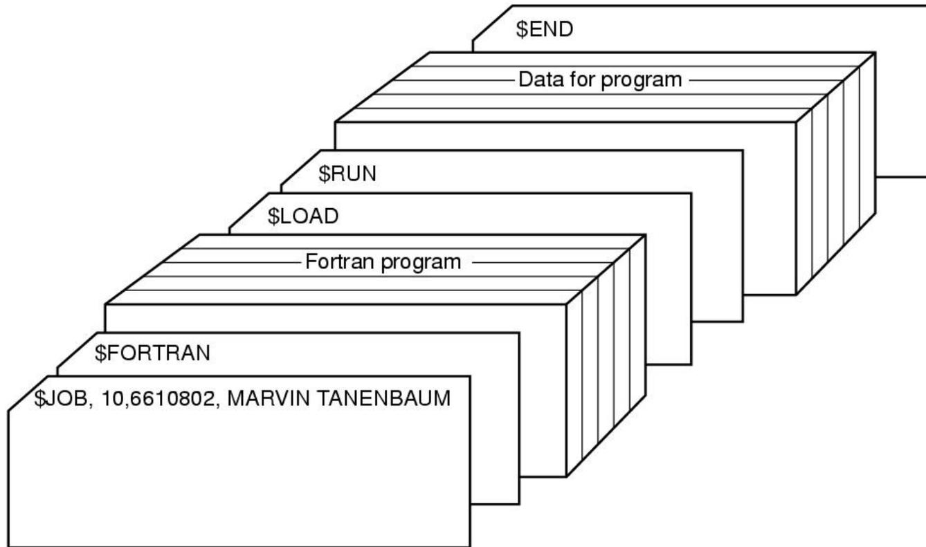
Figure 1-4. Structure of a typical FMS job.
