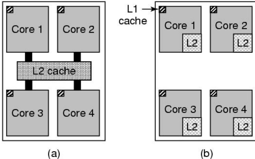
Figure 1-8. (a) A quad-core chip with a shared L2 cache.
