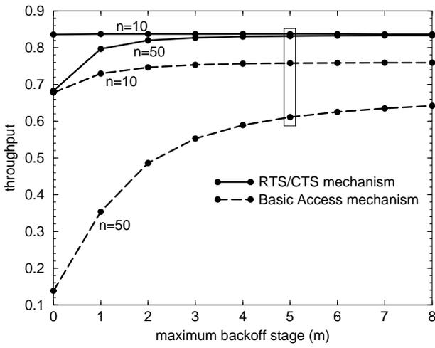
Fig. 13. Throughput versus the maximum number of backoff stages:  $W = 32$
