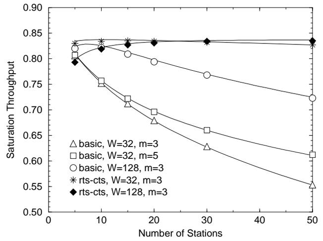
Fig. 6. Saturation Throughput: analysis versus simulation
