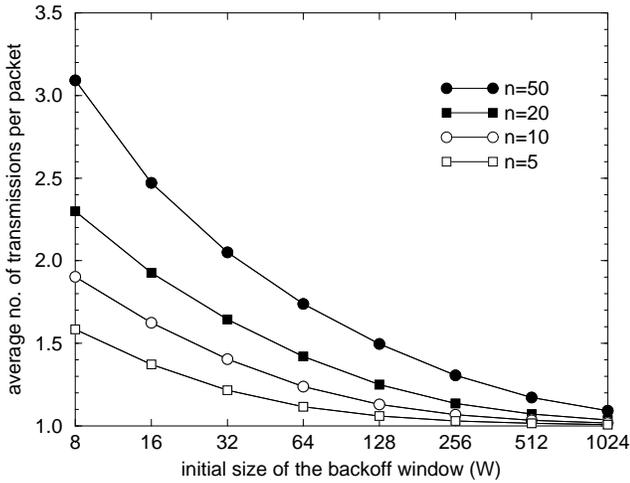
Fig. 14. Average number of transmissions per packet
