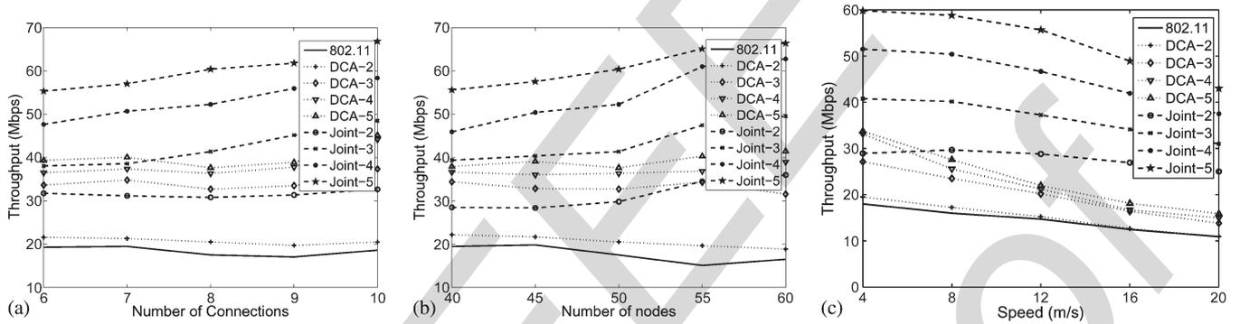
Fig. 8. Throughput for the random topology. (a) Effect of load. (b) Effect of node density. (c) Effect of mobility.
