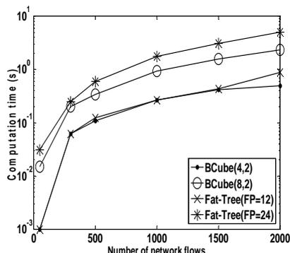
Fig. 16 Computation time of PRA for different numbers of network flows in the BCube and Fat-Tree topologies
