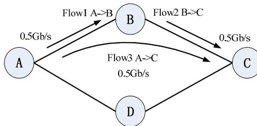
Fig. 1. An example of path assignment with the “incremental” routing algorithm.
