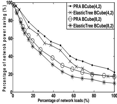
Fig.13 Comparison of PRA with ElasticTree in BCube(4,2) and Bcube(8,2) topologies under the same traffic demand
