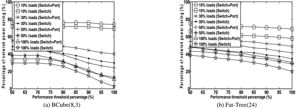
Fig. 8. Network power conservation percentage based on “device-level” and “component-level” granularities under different performance threshold percentages in BCube(8,3) and Fat-Tree(24) topologies.
