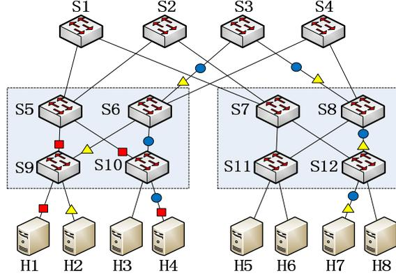
Fig. 4. A path selection example in a partial 4-ary Fat-Tree topology.
