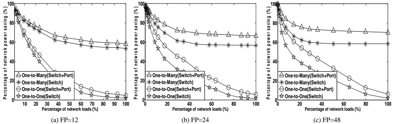
Fig. 10. Network power conservation percentage based on “device-level” and “component-level” granularities under One-to-One and One-to-Many traffic patterns in Fat-Tree topologies.
