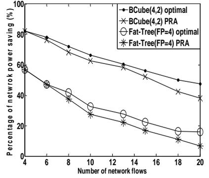
Fig.15 Comparison of PRA with the optimal solution in BCube(4,2) and Fat-Tree(4) topologies under the same traffic demand
