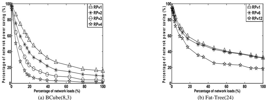
Fig. 12. Network power conservation percentage based on the “component-level” granularity under different reliability requirements in BCube(8,3) and Fat-Tree(24) topologies.
