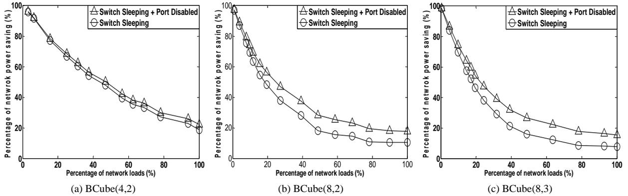
Fig. 6. Network power conservation percentage based on “device-level” and “component-level” granularities under different loads in BCube topologies.
