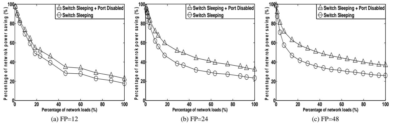
Fig. 7. Network power conservation percentage based on “device-level” and “component-level” granularities under different loads in Fat-Tree topologies.
