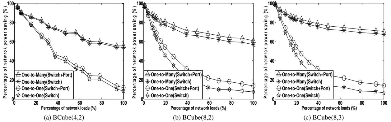
Fig. 9. Network power conservation percentage based on “device-level” and “component-level” granularities under One-to-One and One-to-Many traffic patterns in BCube topologies.
