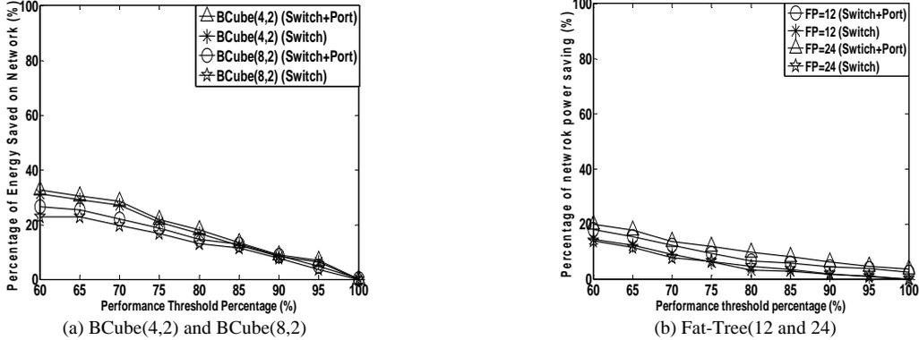
Fig. 11. Network power conservation percentage based on “device-level” and “component-level” granularities under the All-to-All traffic pattern in BCube and Fat-Tree topologies.
