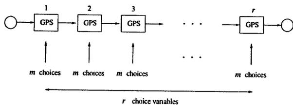
Fig. II.1. End-to-end QoS—given a fixed route—is determined by the local QoS rendered at each of the  $r$  switches which, in turn, is determined by the service class assignment at each switch.
