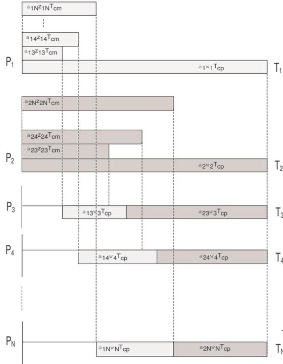
Fig. 3. Timing diagram for a single level tree network with two root processors and concurrent communication.
