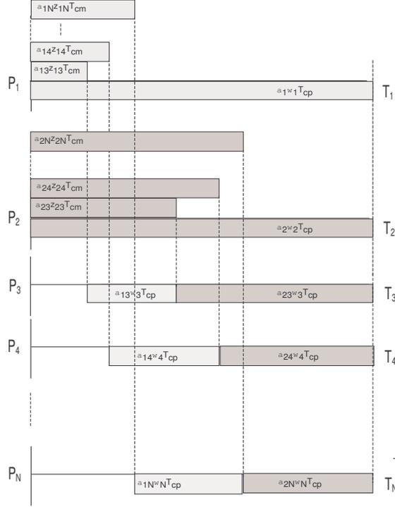
Fig. 4. Timing diagram for a single level tree network with two root processors and concurrent communication : Scheduling for closed form solution.
