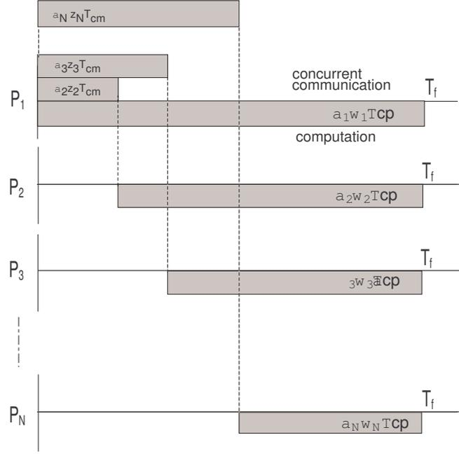
Fig. 2. Timing diagram for a single level tree network with a single root processor and concurrent communication.
