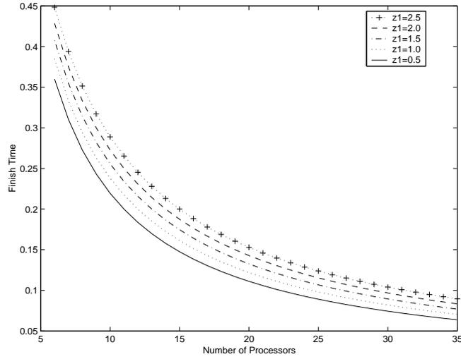
Fig. 5. Finish time versus number of processors, for two root sources single level homogeneous tree network and variable inverse bus speed,  $z_1$ , (first root processor links).
