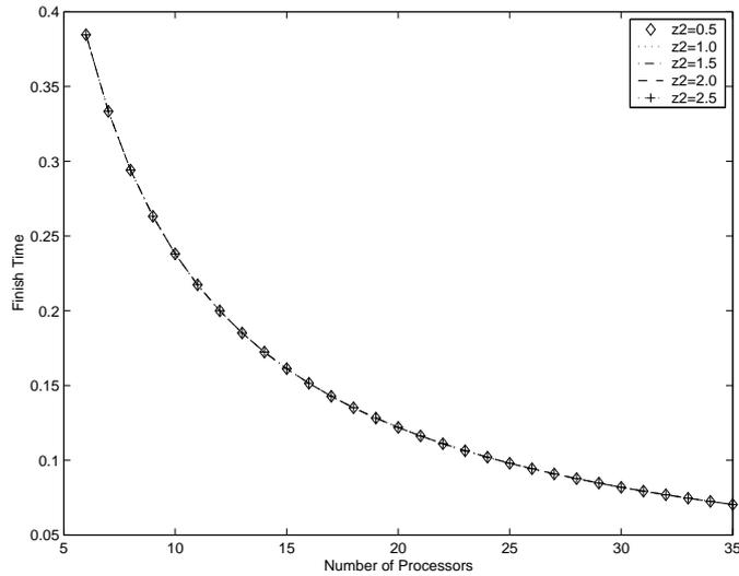
Fig. 6. Finish time versus number of processors, for two root sources single level homogeneous tree network and variable inverse bus speed,  $z_2$ , (second root processor links).
