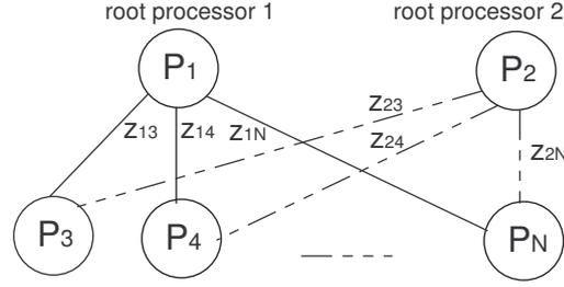
Fig. 1. Single level tree network with two root processors.
