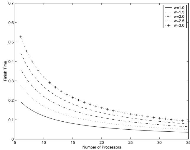
Fig. 7. Finish time versus number of processors, for two root sources single level homogeneous tree network and variable inverse processor speed,  $\omega$ .
