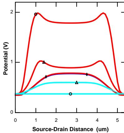
Critical ramping speed is determined by the rate at which the increasing fringing field ( $\sim dV_C/dt$ ) is screened by channel electrons ( $\sim v_{sat}$ )
