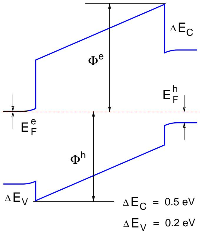
Leakage: holes from collector
