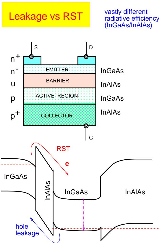
holes injected in the channel recombine non-radiatively
