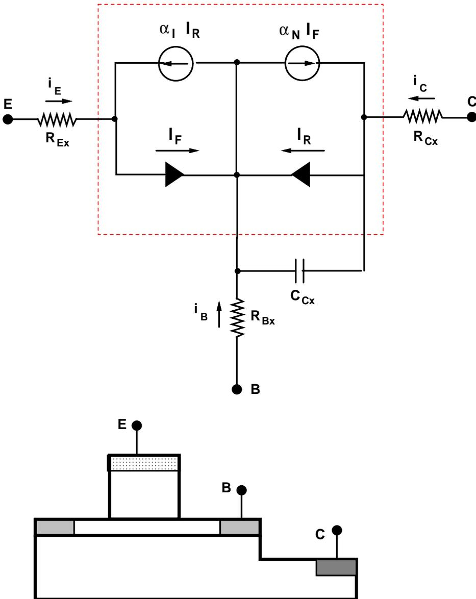
**Figure 1:** Dashed line indicates the "intrinsic" portion of the device, excluding "parasitic" extrinsic elements.
