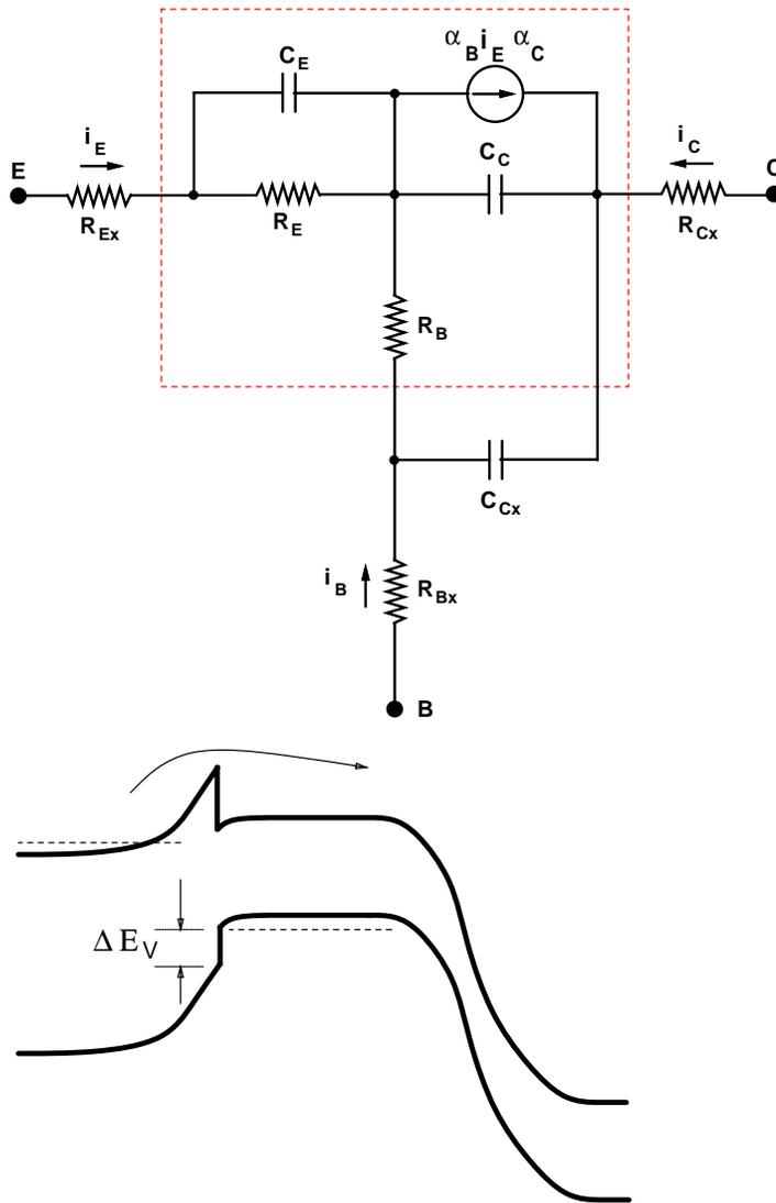
**Figure 2:** This model is good for "ballistic" propagation of carriers across the base. For diffusive propagation, the intrinsic portion must be adjusted,†
