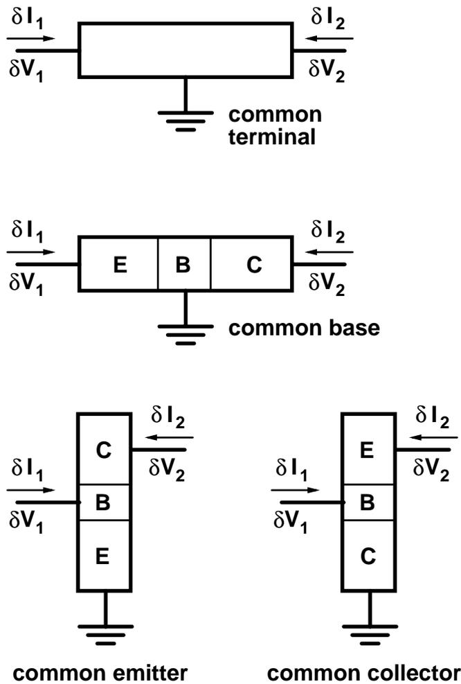
**Figure 4:** Different common-terminal configurations give rise to very different parameters. Thus, the short-circuit current gains are
