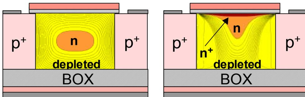
FIG. 1. Cross-section of the  $G^4$ -FET channel. The noise transforms from mobility fluctuations (Hooge) to number fluctuations (McWhorter) when the channel is moved from the volume towards the surface.
