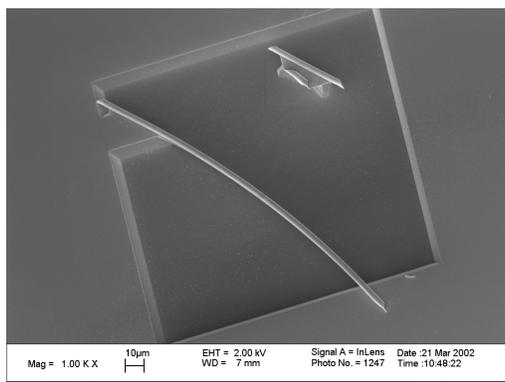
FIG. 1: 230  $\mu\text{m}$  long, free-standing Si/SiGe/Cr nanotube.
