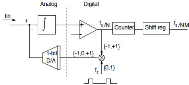
Figure 2: System level diagram of a single channel of the potentiostat.
