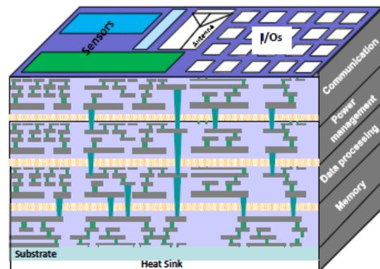
**Figure 1: Monolithic 3-D integration technology where through silicon vias (TSVs) are utilized to achieve communication among the planes.**
