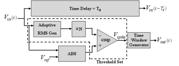
Fig. 3. A block diagram of the adaptive spike detector using absolute value algorithm.
