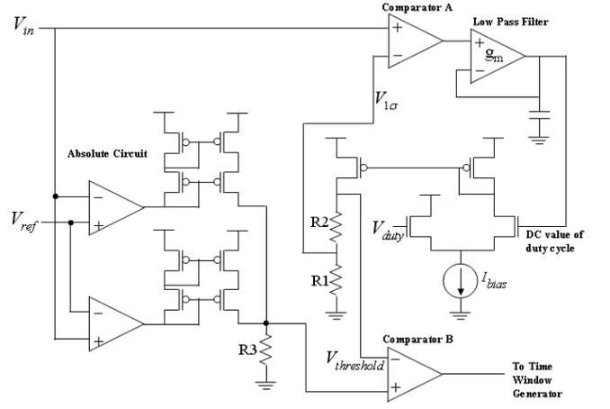
Fig. 6. A schematic of the adaptive spike detector using absolute value. An absolute value circuit was adopted to implement absolute value algorithm and adaptive threshold set scheme was from Harrison's [7], [8].
