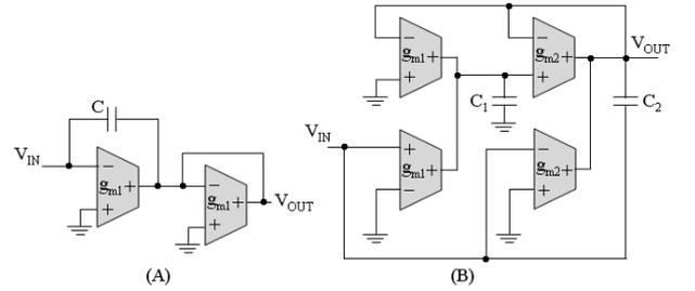
Fig. 7. A first-order (A) and second-order (B) all-pass delay filter circuit.
