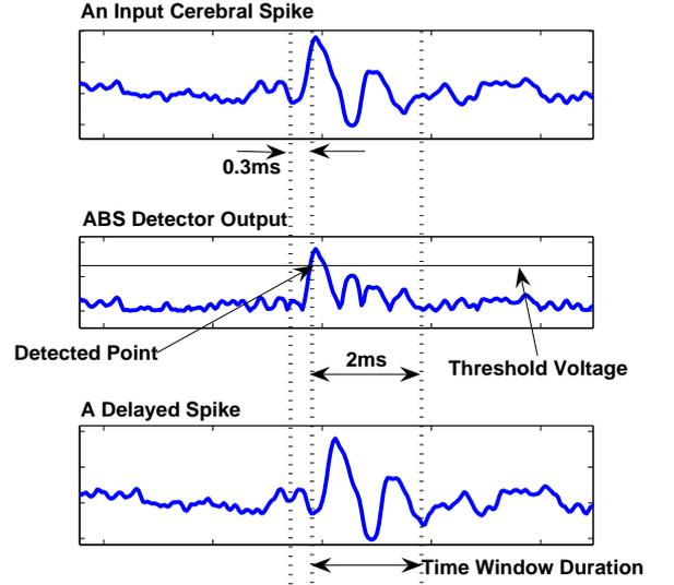
Fig. 4. Typical specifications for a cerebral spike from a rat. This in-vivo data was acquired by Cold Spring Harbor Lab., New York. The threshold value was set by the adaptive spike detection algorithm in MATLAB.
