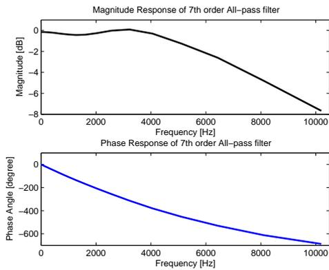
Fig. 8. Magnitude and phase response of simulated 7th-order all-pass filter in Cadence.
