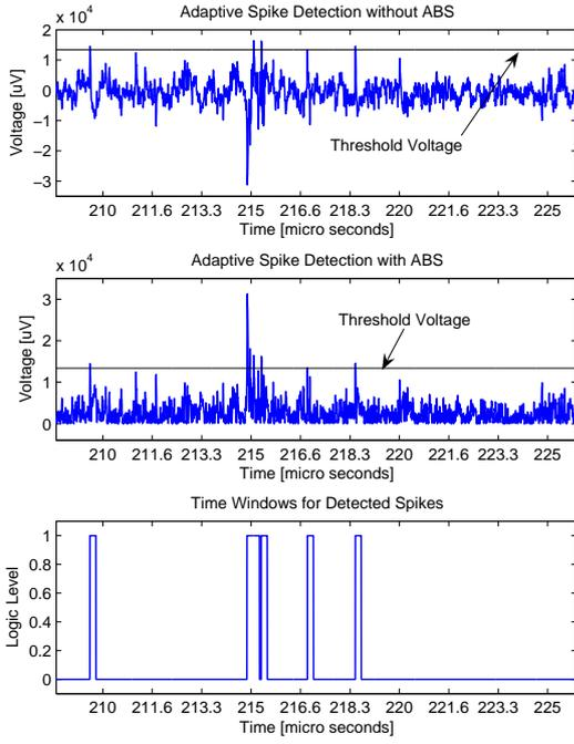
Fig. 5. Comparative views of adaptive spike detector without ABS (figure in the first row) and with ABS (figure in the second row). The detected spikes allow to produce time window signals (figure in the third row).
