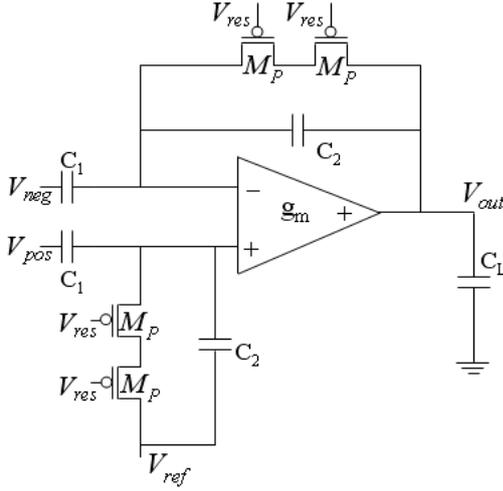
Fig. 2. Schematic diagram for a low-input-referred-noise pre-amplifier.
