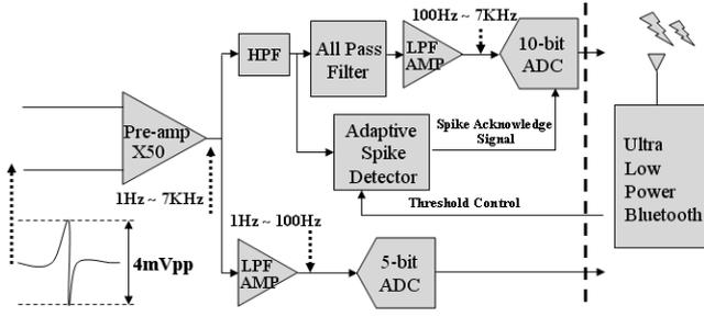
Fig. 1. A single-channel system diagram for the proposed adaptive neural recording system.
