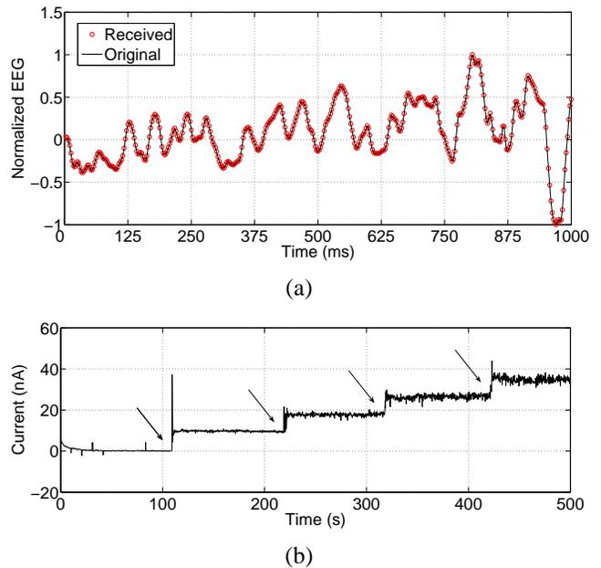
Fig. 3. (a) Original and demultiplexed LFP data shown for a 1 second window. (b) Demultiplexed output of one potentiostat channels showing response to the addition of the neurotransmitter dopamine to the test solution.
