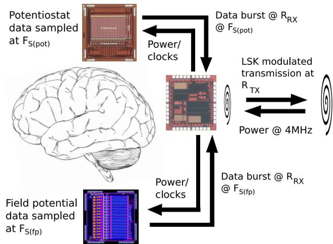
Fig. 1. System diagram showing the individual chips with variable data rates in an eventual implantable scenario. In this work the field potential data is played from a memory.
