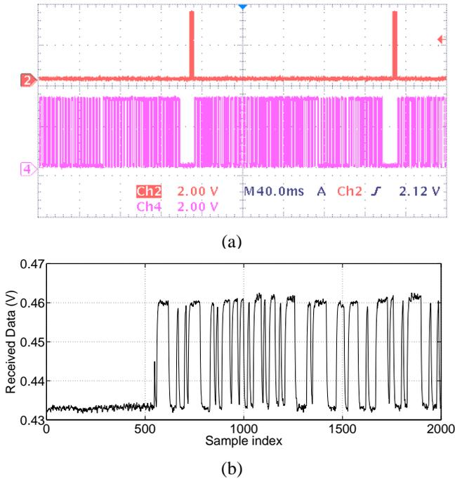
Fig. 2. (a) Scope plot showing the timing of our scheme. The top trace is the potentiostat data burst. Lower trace shows the transmission of the multiplexed potentiostat and field potential data. (b) Shows a portion of the data received at the base station after demodulation with a peak follower.
