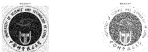
Figure 11. Extracted watermarks after JPEG compression of watermarked baboon with ratio 1.7 (left) and 2.3 (right)
