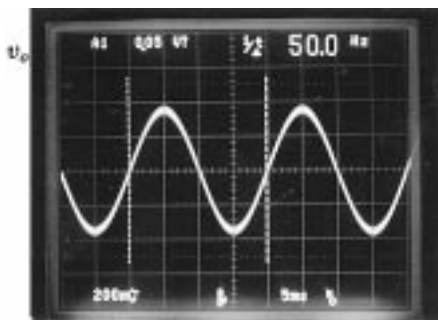
Fig. 5. Output voltage waveform in the closed-loop dc-ac power inverter. Horizontal scale: 5 ms/div.; vertical scale: 0.2 V/div.
