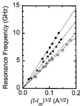
Fig. 3. RIN maximum frequency versus square root of pumping current for FP (triangles) and DFB (circles) devices at 25 °C. Open and solid symbols represent data for moderately and heavily doped lasers, respectively.
