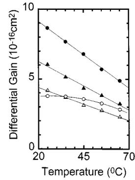
Fig. 4. Temperature dependence of the differential gain for moderate (open symbols) and heavy (solid symbols) doping for FP (triangles) and DFB (circles) lasers.
