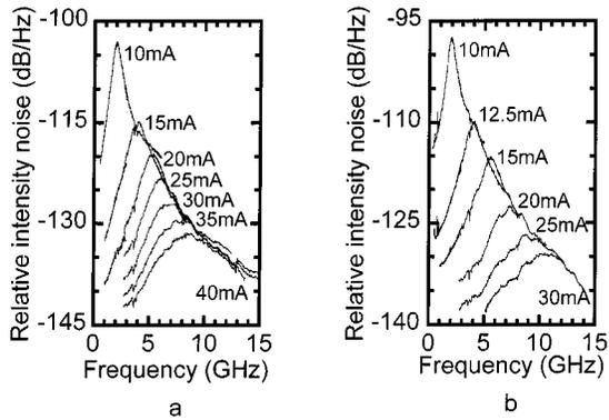
Fig. 2. RIN spectra at different bias currents (a) for moderately doped and (b) for heavily doped DFB devices at 25 °C.
