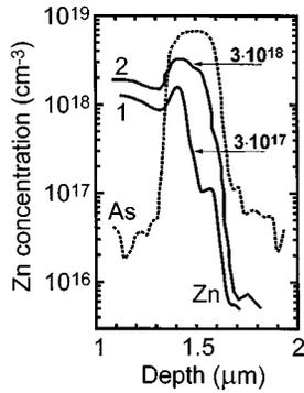
Fig. 1. SIMS data for (1) moderately and (2) heavily doped structures. The As signal shows the position of the active region.
