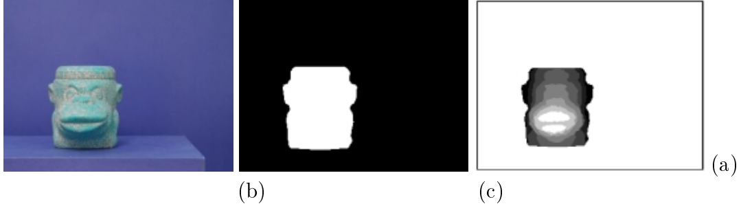
Figure 2.8: An example of object segmentation and stereo matching (a)An image of a stereo pair (b)Segmented object (c) Stereo matching result on segmented region
