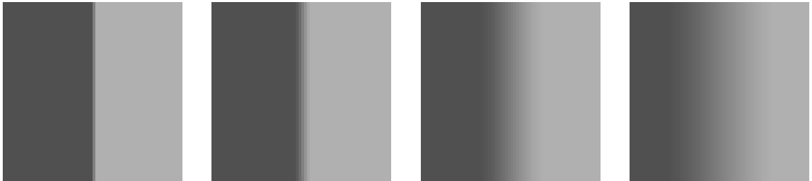
Figure 4.2: Step edge focused at step 0 and defocused images at lens steps 10,40,70
