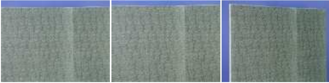
Figure 2-24: Test objects with random pattern are used for planar fit
